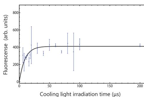
**Figure 5.** Variation in total fluorescence when changing the cooling light irradiation time. Curve is fitted considering the number of atoms decay exponentially. The resultant lifetime was 10  $\mu s$ .
