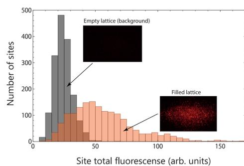
**Figure 4.** Fluorescence intensity histogram of atoms trapped in the two-dimensional optical lattice measured over 1620 sites. Black: empty lattice (background) histogram and orange: center portion of a filled lattice histogram.
