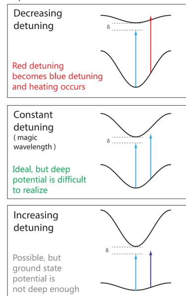
Increasing detuning lattice with Yb can be created using a lattice wavelength near resonant to the excited  $^1P_1 \rightarrow (6s7s)^1S_0$  transition.
