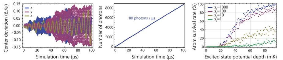
**Figure 1.** Simulation of an atom trapped in a two-dimensional optical lattice with an incident cooling light. Left: Deviation of the atom in each direction  $\Delta$  relative to the lattice spacing  $a$ . Middle: Number of spontaneous emissions due to the incident cooling light. Right: Percentage of atoms that remain trapped after 100 $\mu s$  for different lattice potential depths.  $s_0$  is the saturation intensity of the cooling light.
