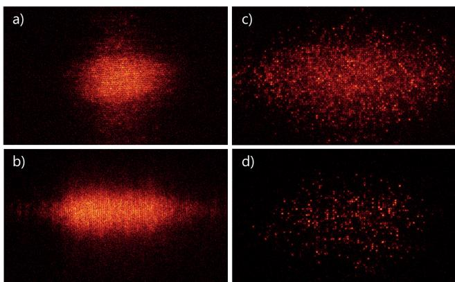
**Figure 2.** (False color) Typical fluorescence raw images of the atoms trapped in the optical lattice. a) One-dimensional optical lattice in the horizontal and vertical (x and y) directions. b) Fluorescence in the case of a filled lattice and d) sparse filled two-dimensional optical lattices.
