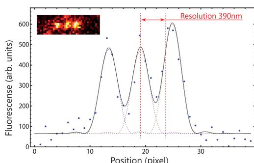
**Figure 3.** Intensity profile through the center axis of the image generated by three consecutive sites. The airy function fitting shows a resolution of 390 nm. The expected resolution for our microscope system with a NA of 0.8 is 270 nm.
